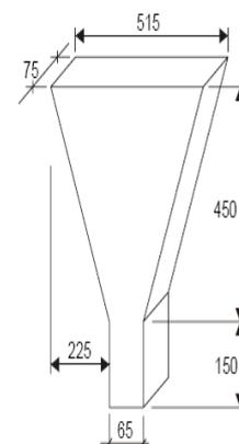
Fig. 3.3: V-funnel apparatus
