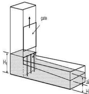
Fig. 3.2: L-Box Apparatus
