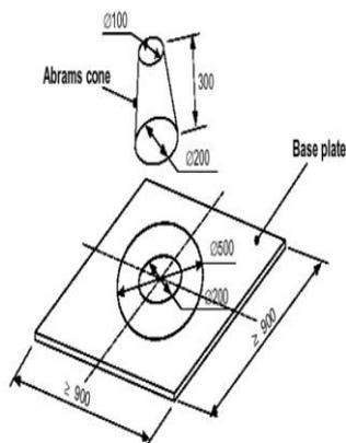
Fig. 3.1: Base plate and Abrams cone
